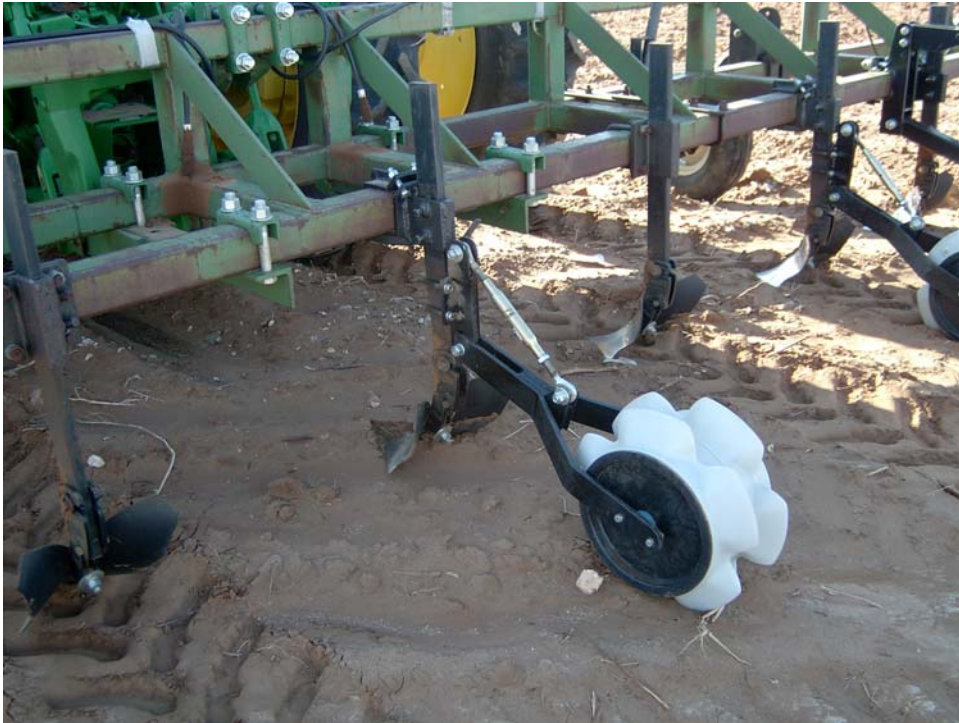
Figure 1—Photo of the imprinter unit installed behind busters
